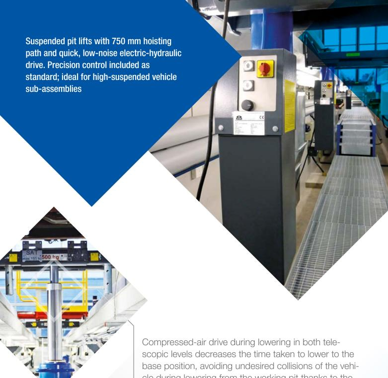
cle during lowering from the working pit thanks to the piston rod that always retracts
